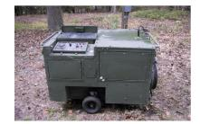
Description: The IASH (H-140) is a multi-fueled, powered heater that provides a maximum heat output of 140K BTU. Operates in an ambient temperature range from -60°F to 100°F and burns JP-8, DF-1, DF-2, and DF-A fuels for up to 8 hours unattended on a 14-gallon internal fuel tank. Safety features include an automatic shutdown in the event of an over temperature condition if the heater overheats or detects carbon monoxide gas in the shelter or return airflow.
